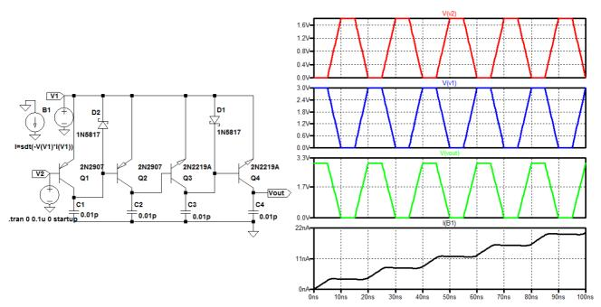
Recovered-energy logic (REL) inverter circuits diagram and waveforms
