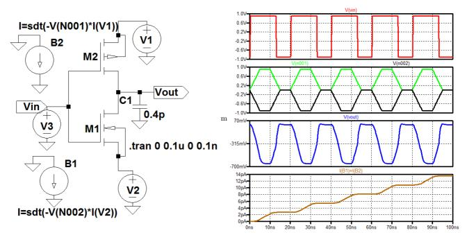
${\bf Fig.\,2} \quad \text{ Split level pulse 1n1p logic inverter circuits diagram and waveforms}$
