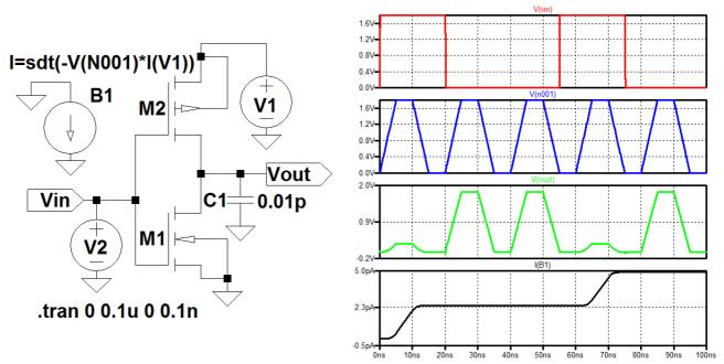
1n-1p quasi-adiabatic logic inverter circuits diagram and waveforms
