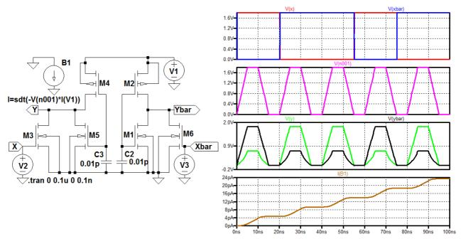
Fig. 5 2n-2n2p quasi-adiabatic logic inverter circuits diagram and waveforms
