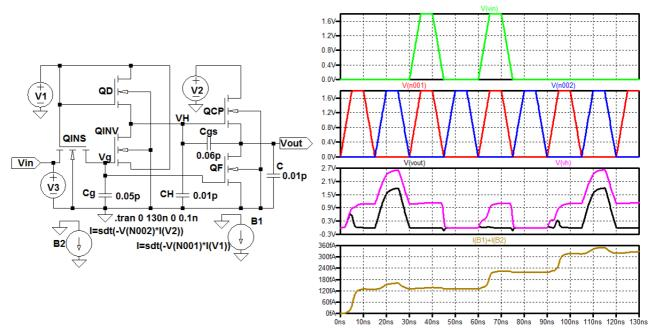
${\bf Fig.\,6} \quad \ {\rm Hot\text{-}clock\ nMOS\ logic\ inverter\ circuits\ diagram\ and\ waveforms}$
