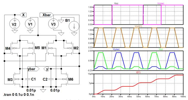
${\bf Fig.\,1} \quad \ \ {\bf 2n2p\text{-}2n \ adiabatic \ logic \ inverter \ circuits \ diagram \ and \ waveforms}$
