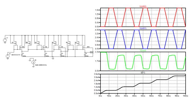
Fig. 8 Recovered-energy logic (REL) in MOSFETs inverter circuits diagram and waveforms
