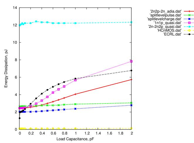
Fig. 11 Energy dissipation comparison in adiabatic circuits at different load capacitance  $\,$ value
