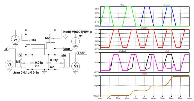
Fig. 10 Efficient charge-recovery logic (ECRL) circuits diagram and waveforms
