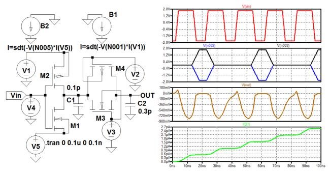
Split level charge-recovery logic inverter circuits diagram and waveforms
