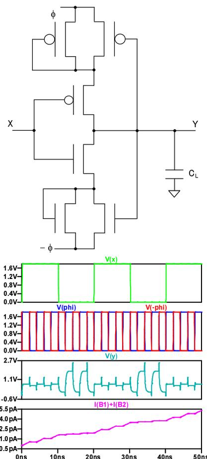
**Fig. 1** Quasi-static energy recovery logic (QSERL) circuit diagram and waveforms
