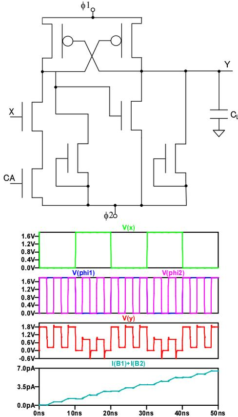
**Fig. 2** Adiabatic pseudo-domino logic (APDL) circuit diagram and waveforms
