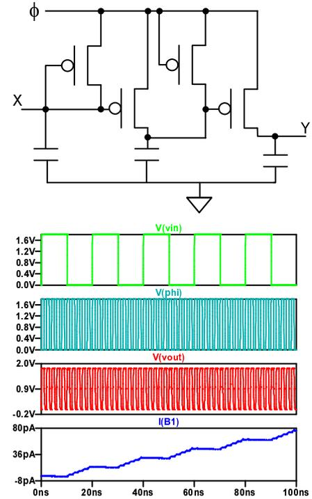
**Fig. 3** Recovery energy logic (REL) circuit diagram and waveforms
