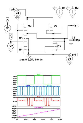
$\label{eq:Fig.4} {\bf Fig.4} \quad {\rm Recovery\ energy\ logic\ (REL)\ circuit\ diagram\ and\ waveforms}$
