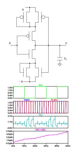
Quasi-static energy recovery logic (QSERL) circuit di-Fig.1 agram and waveforms
