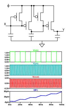
$\label{eq:Fig.3} {\bf Fig. 3} \quad {\rm Recovery\ energy\ logic\ (REL)\ circuit\ diagram\ and\ waveforms}$
