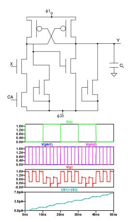
$\label{eq:Fig.2} {\bf Fig.2} \quad {\rm Adiabatic\ pseudo-domino\ logic\ (APDL)\ circuit\ diagram\ and\ waveforms$
