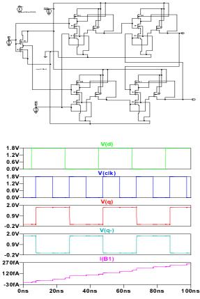
Fig. 5 Simulation output waveforms of clocked D (Data) flip-flop of CMOS.
