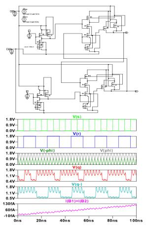
Fig. 4 Simulation output waveforms of SR (set-reset) flip-flop of 2PASCL.
