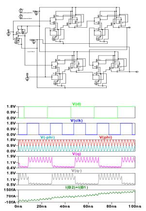
Fig. 6 Simulation output waveforms of clocked D (Data) flip-flop of 2PASCL.
