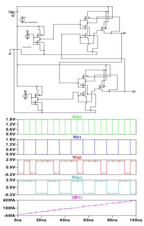
Fig. 3 Scheme and output waveforms of SR (set-reset) flip-flop of CMOS from the simulation.
