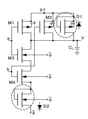
Fig. 2 Leg 2: NAND logic circuit with 2PASCL configuration. nMOS bulk connected to  $\overline{\phi}$  and pMOS bulk to  $\phi$ .
