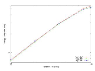
Fig. 4 NAND logic energy dissipation comparison between leg 1,2 and 3.
