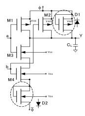
Fig. 3 Leg 3: NAND logic circuit with 2PASCL configuration. nMOS bulk connected to Vss and pMOS bulk to Vdd.
