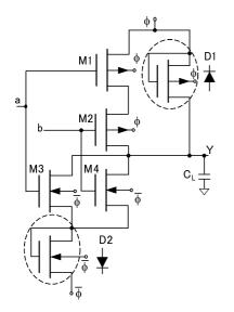
Fig. 3 NOR logic circuit with 2PASCL configuration. nMOS bulk connected to  $\overline{\phi}$  and pMOS bulk to  $\phi$ .
