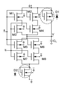
Fig. 4 exclusive-OR logic circuit with 2PASCL configuration. nMOS bulk connected to  $\overline{\phi}$  and pMOS bulk to  $\phi$ .
