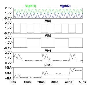
Fig. 5 2PASCL NOR logic circuit with sinusoidal driving voltage.
