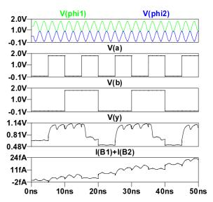
Fig. 6 2PASCL exclusive-OR logic circuit with sinusoidal driving voltage.
