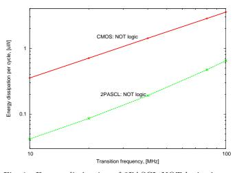
Fig. 1 Energy dissipation of 2PASCL NOT logic circuit compared to CMOS.
