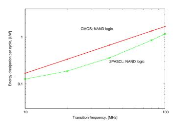
Fig. 2 Energy dissipation of 2PASCL NAND logic circuit compared to CMOS.
