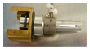
Fig. 12. Round heater element mounter
