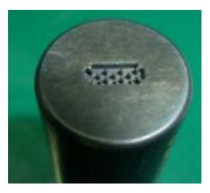
Fig. 10.Ejectorless cavity
