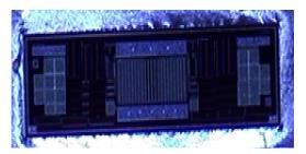
Fig. 2. High aspect ratio die 32 mils x 125 mils
